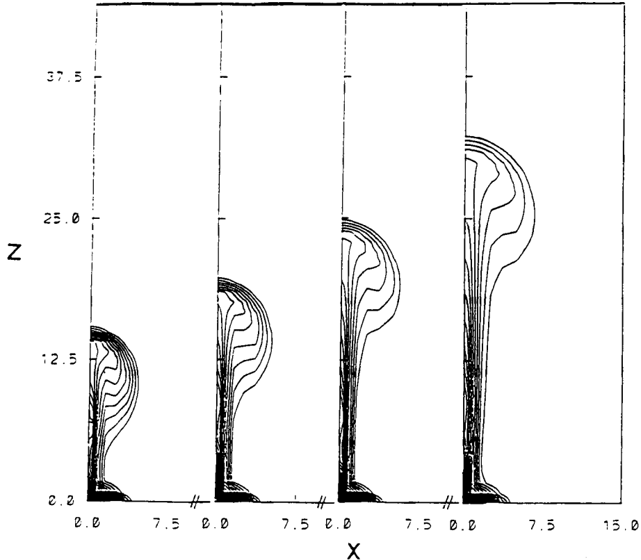
Figure 8. Snapshots of the plume temperature contours for the T_{\text{amb}} = 0.1 °C plume case for four times, 1.5, 2.0, 2.5 and 3.1 h (from left to right). Axis lengths are non-dimensional (using the new scaling of Section 6) and are to be multiplied by a factor of 1.58 to get real dimensions. Only about one-third of the total width of the model is shown
